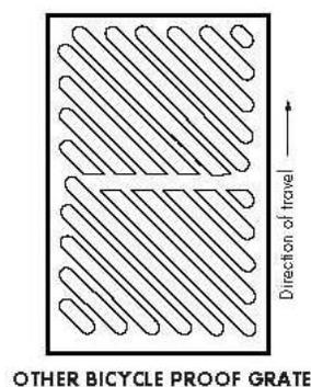
On roadways with shoulders, the grate should be placed outside the travel path of the bicyclist, i.e. 48 inches of clear pavement should be maintained between the shoulder stripe and the left edge of the drainage grate. If 48 inches cannot be provided within the existing shoulder width, the shoulder can be widened to accommodate the grate, with the taper on the outside edge, or a narrower grate should be selected. See also Section 7.4.2 and Figure 7-13.
