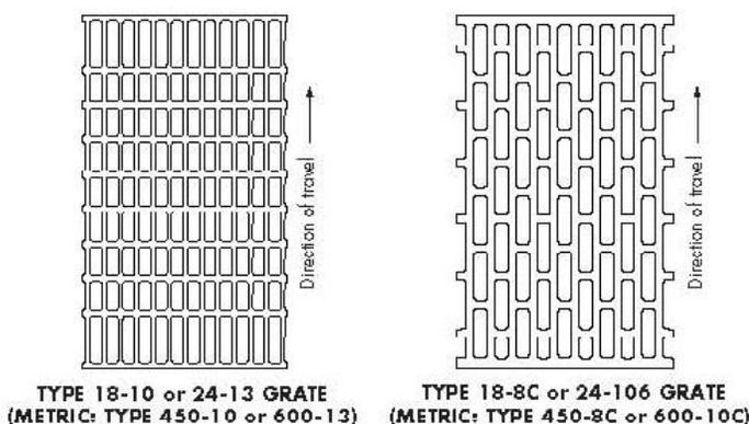
Optimally the roadway should be designed so that the bicyclist does not have to traverse the grate per HDM Section 837.2. On roadways with curb and gutter, the grate should not be wider than the gutter pan. If the gutter pan needs to be widened to accommodate a large drainage grate, the taper should be on the outside edge.
