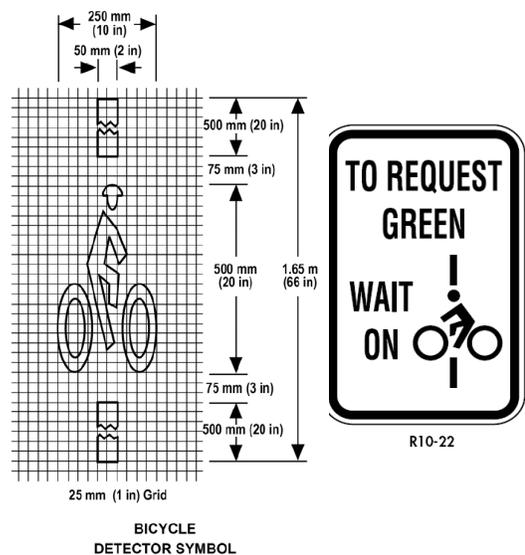
Inductive loops are still the most common technology employed. Two types of inductive loop detectors are typically used; the Diagonal Quadrupole Loop – Type “D” is typically used in vehicle lanes, and the Quadrupole Loop – Type “C” is typically used in bike lanes. The bicycle detection symbol may be used to show a bicyclist where to stop in a bike lane or traffic lane to be detected.
